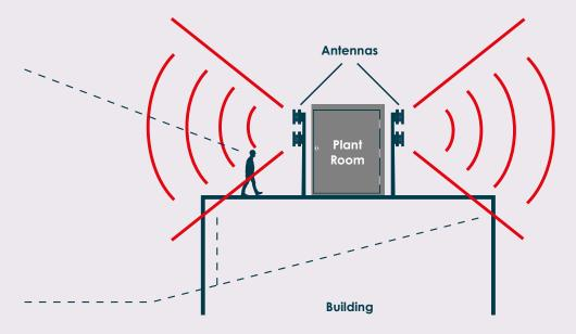
Each Scenario is indicative and a simplified version to demonstrate the technical constraints and solutions. Although 2D was used for simplicity, antennas must be carefully sited at locations on a building to provide 360 degree coverage, and must always be ICNIRP compliant.
