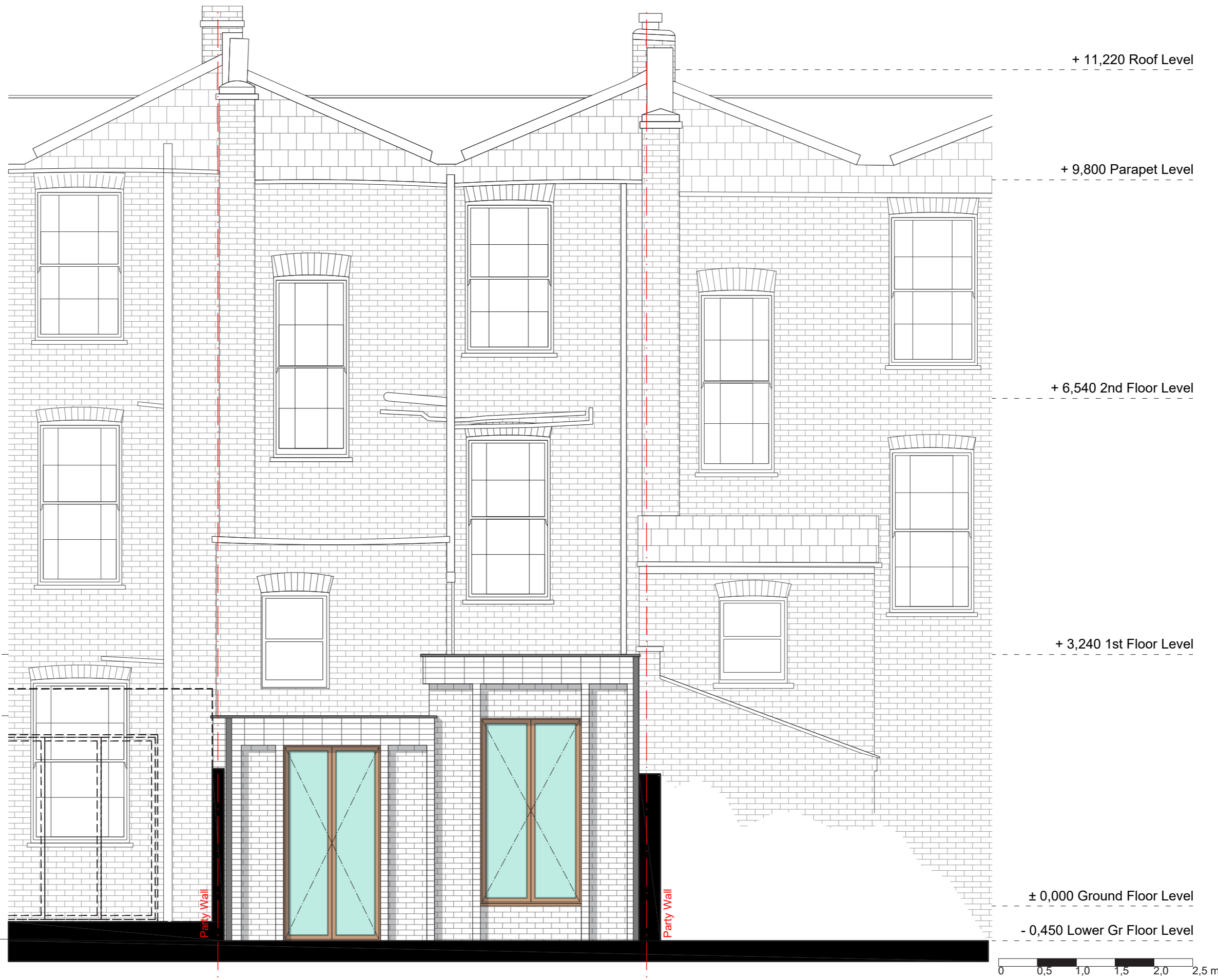
013 01 Proposed Rear Elevation Scale 1:50 @ A3 / 1:25 @ A1
