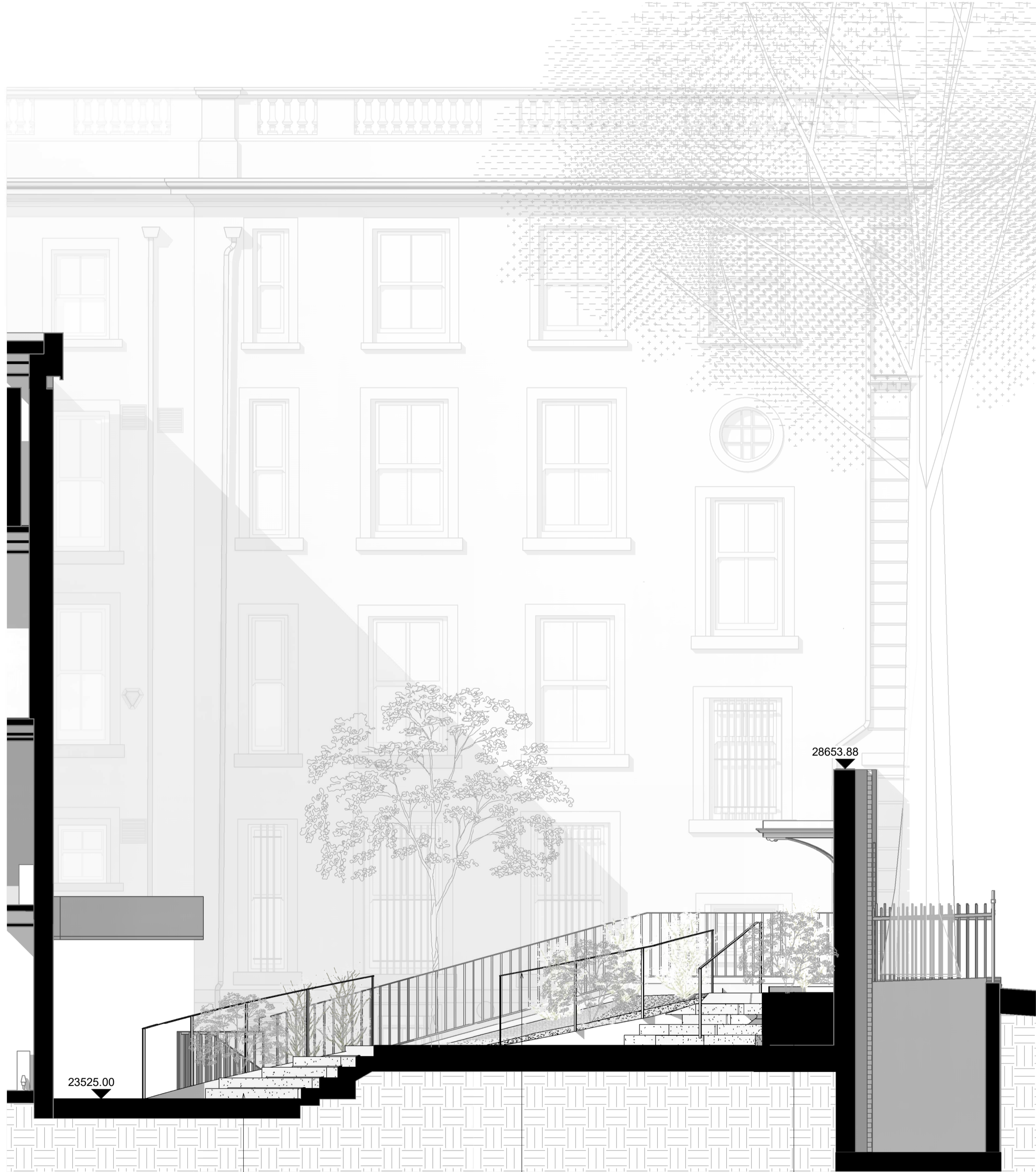
Proposed Garden Section 1 : 50 STONE STEPS METAL BALUSTRADE TIMBER CLADDED SEATING AREA AND RAISED PLANTER BED
