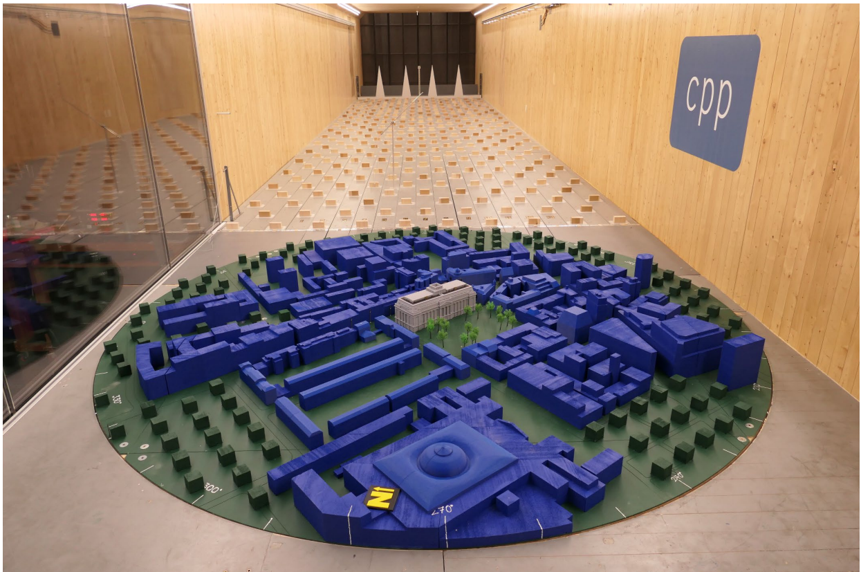
Figure 4: Rendering of the wind tunnel used for testing and photograph of the wind-tunnel configuration. Note spires and trip at entrance to test section, and roughness elements on approach fetch to develop a turbulent boundary-layer flow.
