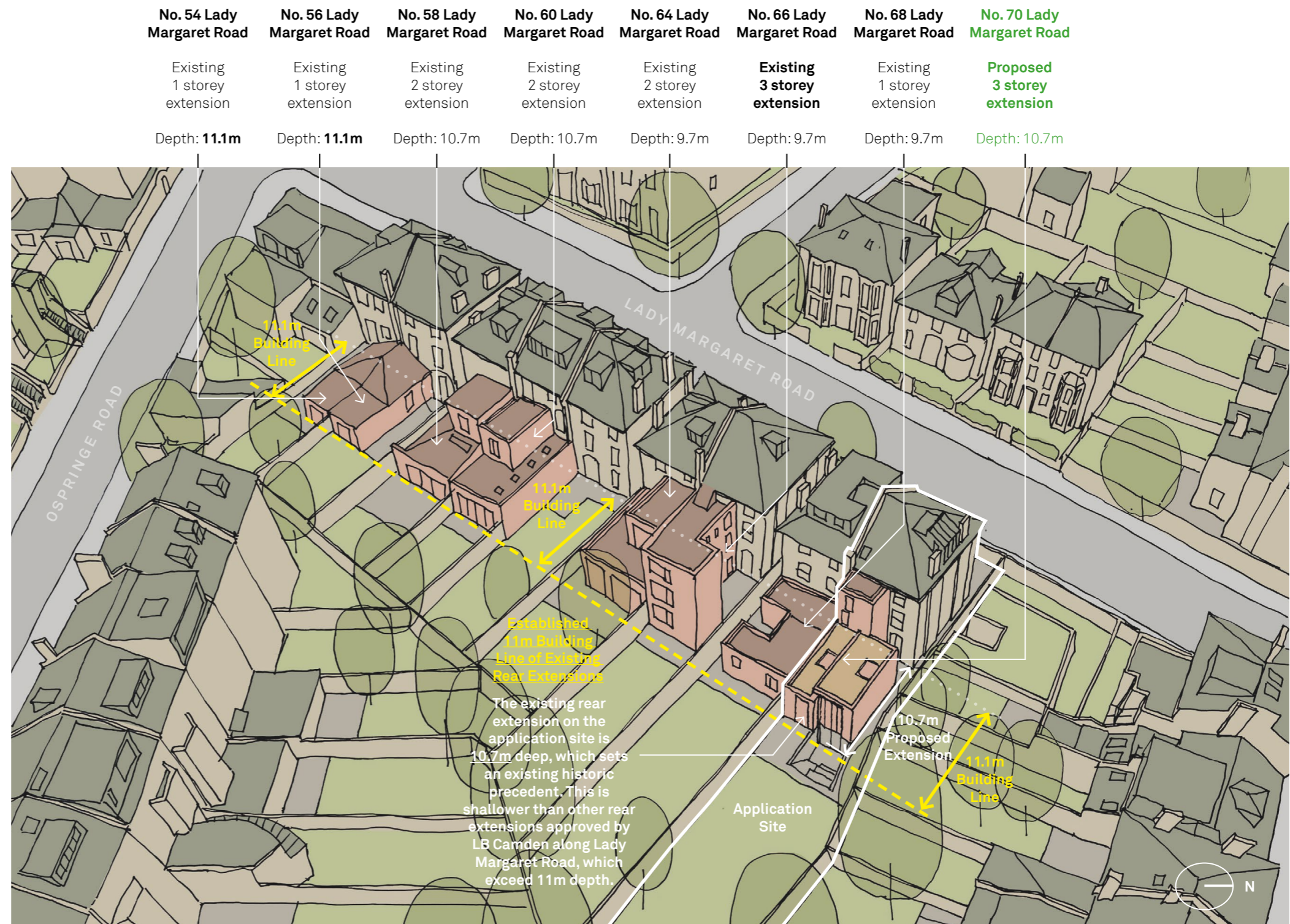
Proposed Replacement Extension within with Established Building Line of Existing Rear Extensions along Lady Margaret Road
