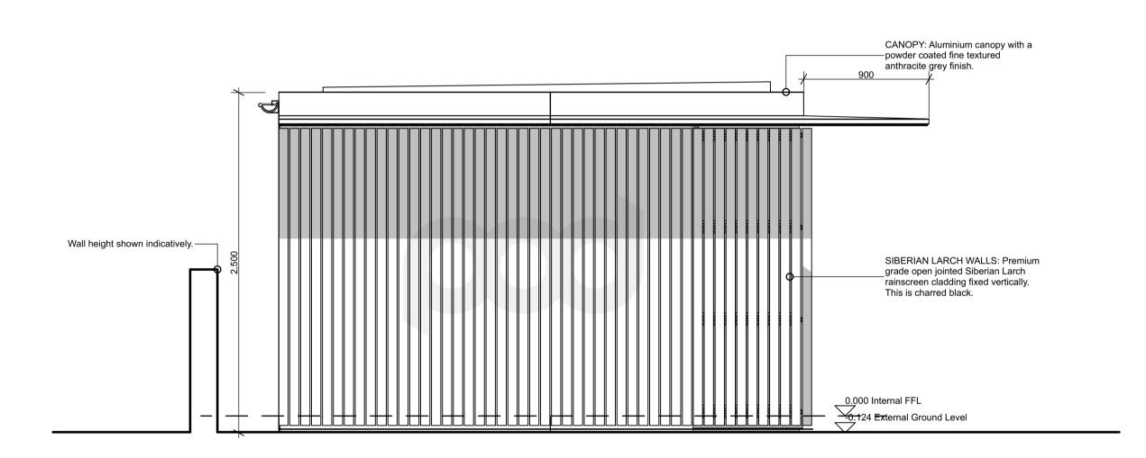
1:25 E-03 Elevation E-04 Elevation 1:25
