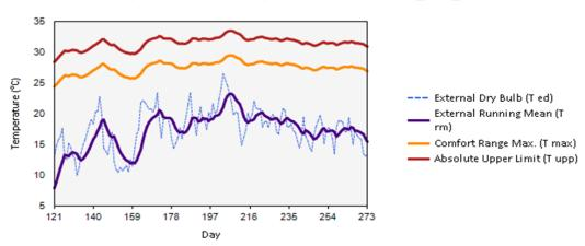
The adaptive overheating assessment tests rooms against three criteria. If a room fails any two of the three criteria, then it is said to overheat.
