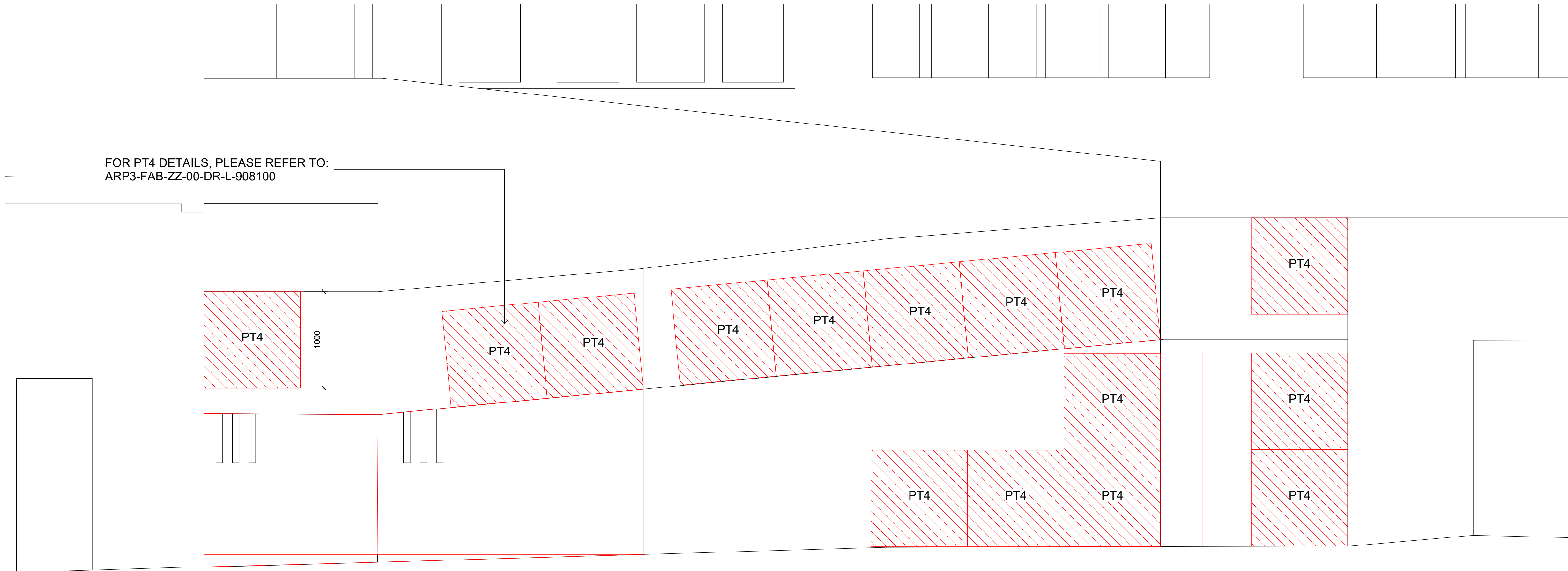
2 DETAILED ELEVATION - Salvaged Precast Concrete Panel Cutting Schedule 1 : 25
