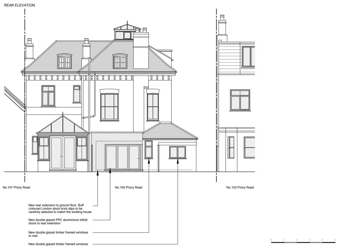
Rear elevation drawing showing the proposed new rear extension to Flat 1 and the existing rear extension to Flat 3.
