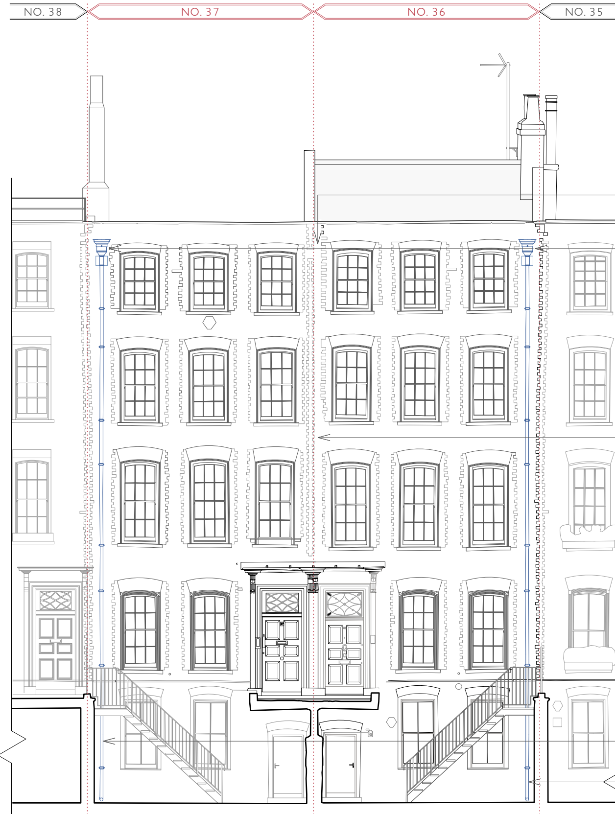
PROPOSED FRONT ELEVATION @ 1: 100 PROPOSED RE-INSTATEMENT OF THE RAIN WATER PIPES AND HOPPERS
