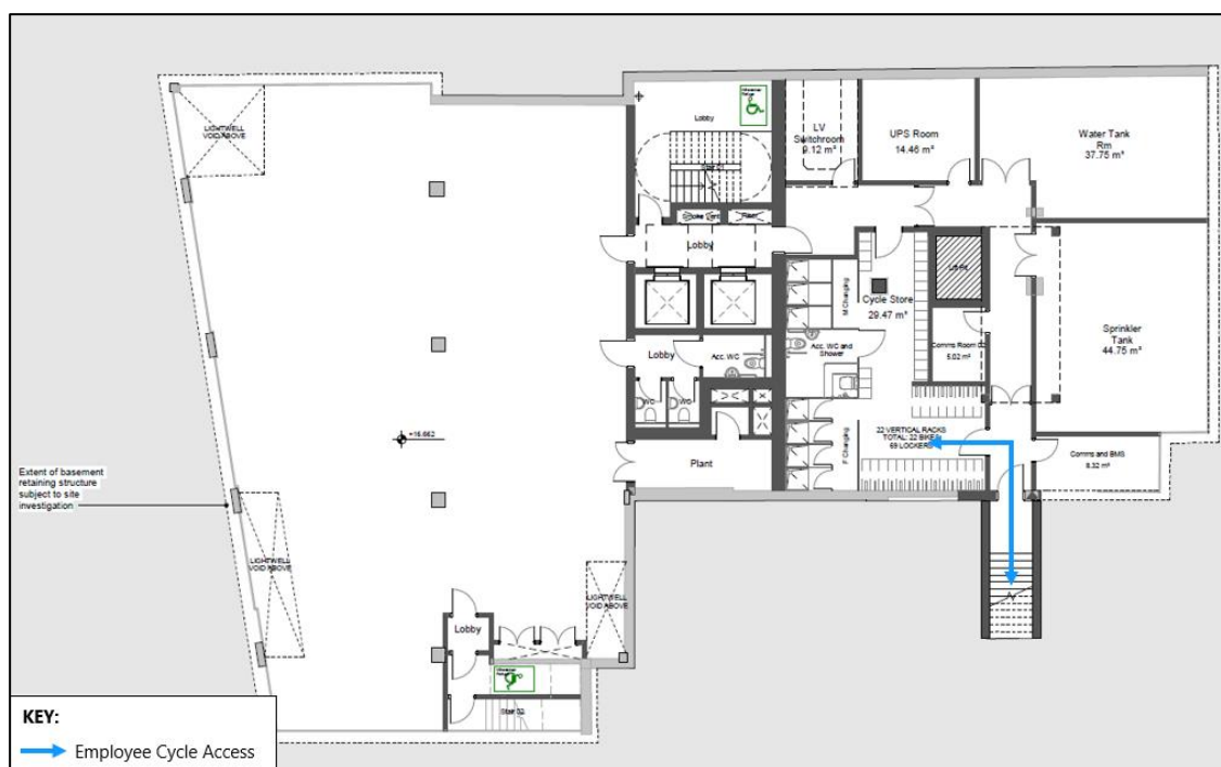
Figure 5.2: Basement Cycle Access
