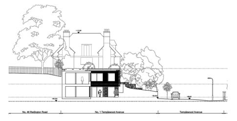
Proposed formation level for the development is understood to be at about 98.5 m OD. Therefore, whilst proposed lower ground floor level will be at a similar elevation to the adjoining street on the southern part of the site, it will extend to a depth of about 4.5 m to 5.0 m beneath the level of the adjoining garden on the northern part of the site.
