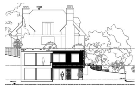
It is understood from information provided by Conisbee, that the majority of excavations for the new structure will be supported by a contiguous bored pile wall, with new RC retaining structures proposed on the southern part of the site to replace the existing brick structures.
