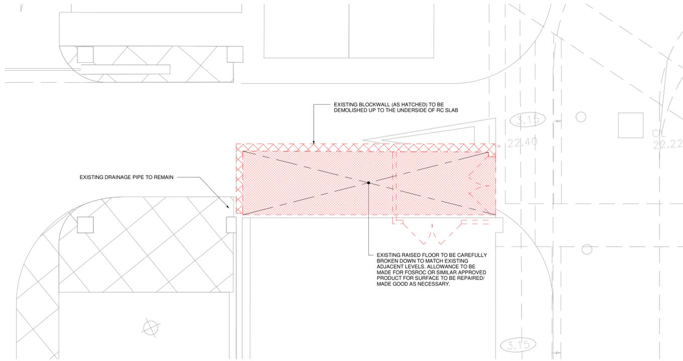
1. PART BASEMENT PLAN SHOWING WALL/FLOOR TO BE DEMOLISHED
