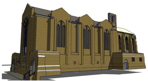
Above: sketch-up model of the church with south chapel to the far-right – the leadwork making a slightly heavier line over the top edge of the parapet.
