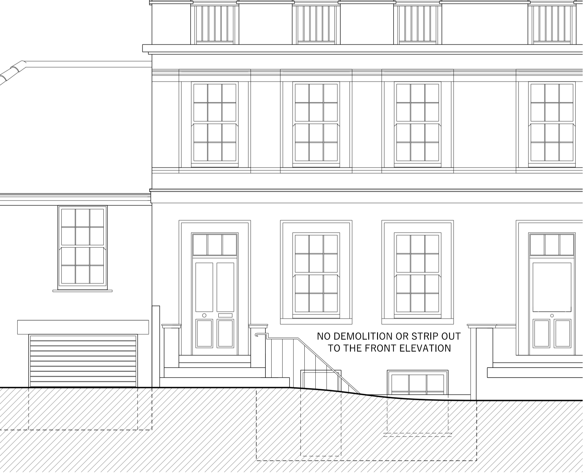
Proposed Front Elevation - Demolition Drawing
