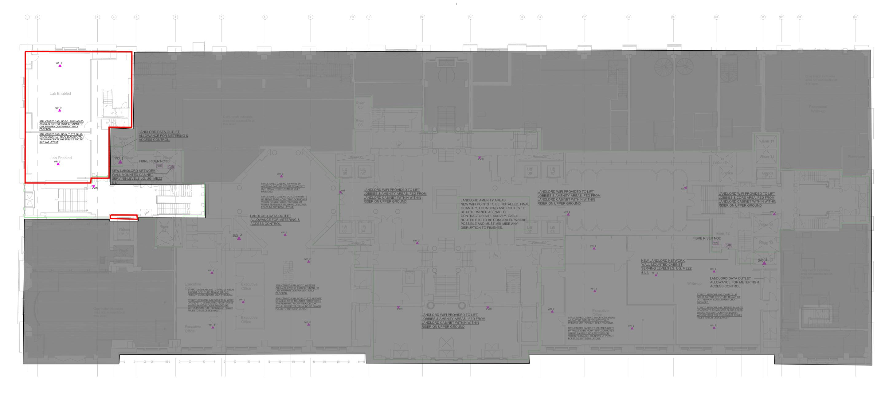
DATA CABLING FROM PRIMARY ROUTES TO OUTLETS SHALL BE ROUTED IN CONDUIT OR ON TRAY/BASKET. FINAL ROUTES TO BE DETERMINED ON SITE. CABLE ROUTES SHALL BE CONCEALED WHEREVER POSSIBLE.
