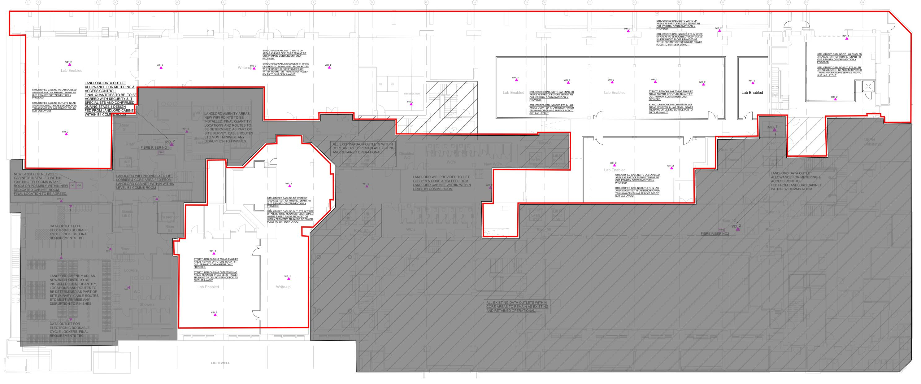
DATA CABLING FROM PRIMARY ROUTES TO OUTLETS SHALL BE ROUTED IN CONDUIT OR ON TRAY/BASKET. FINAL ROUTES TO BE DETERMINED ON SITE. CABLE ROUTES SHALL BE CONCEALED WHEREVER POSSIBLE.
