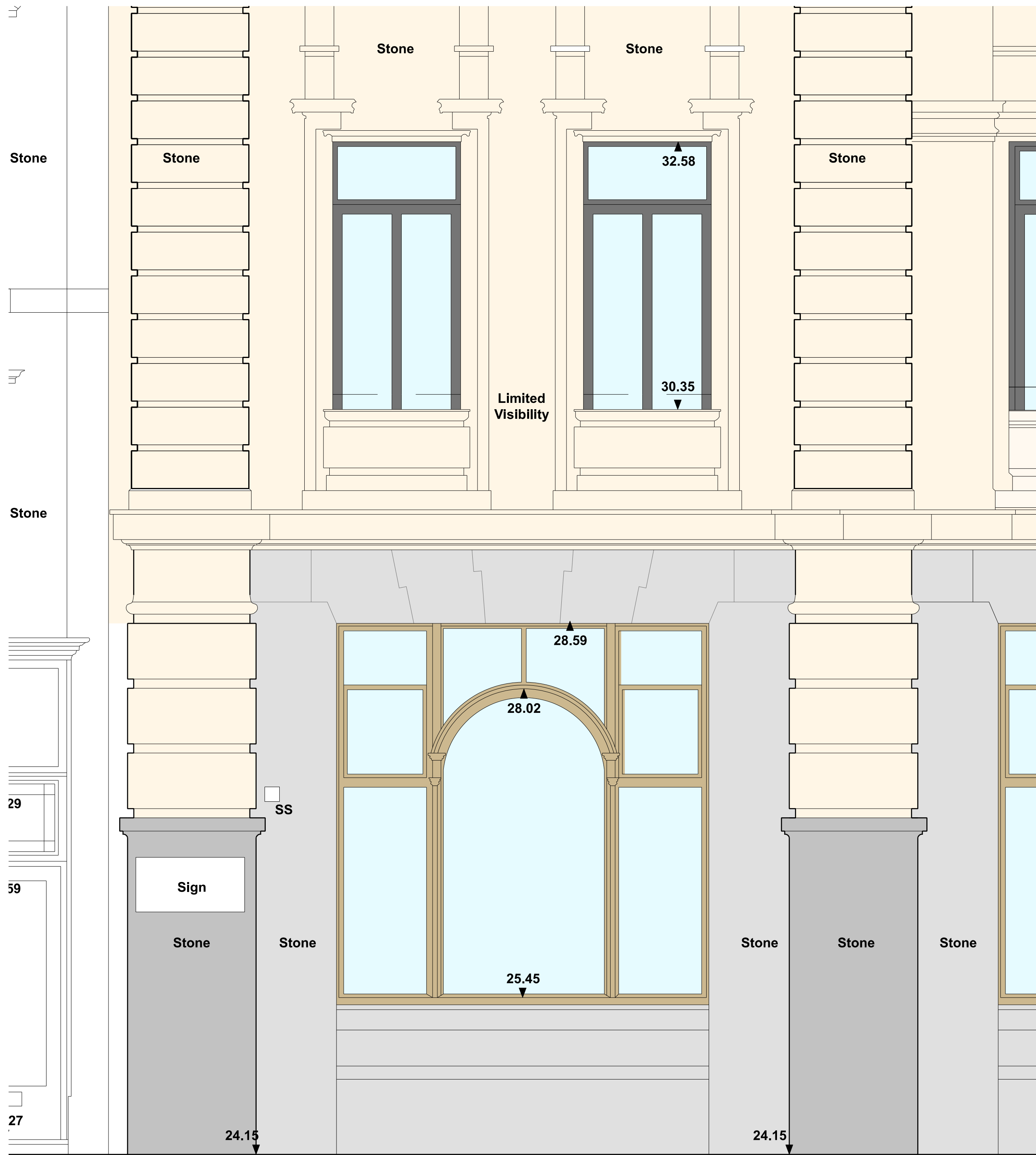
Typical Bay Elevation 01 748-19040
