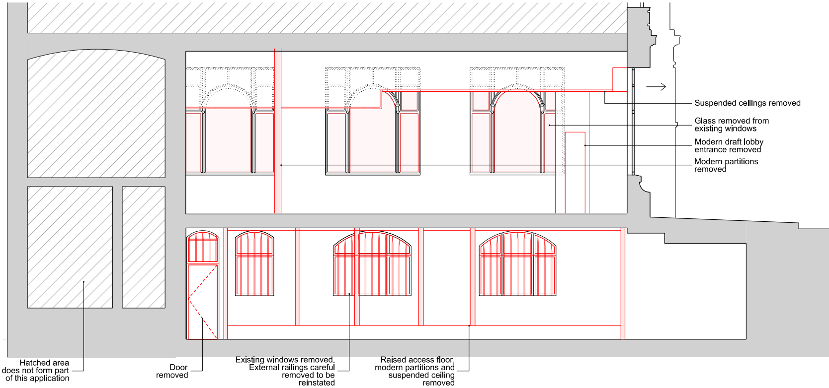
Existing with proposed demolition Section DD
