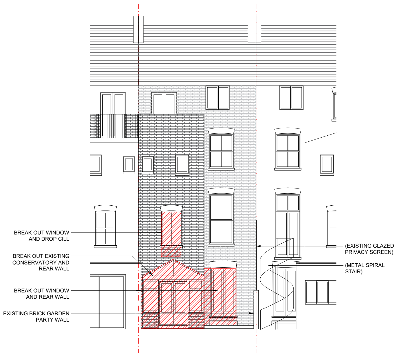
xAA EXISTING ELEVATION AA 0 0.5 1 2 3 1:50 at A1 DEMOLITION
