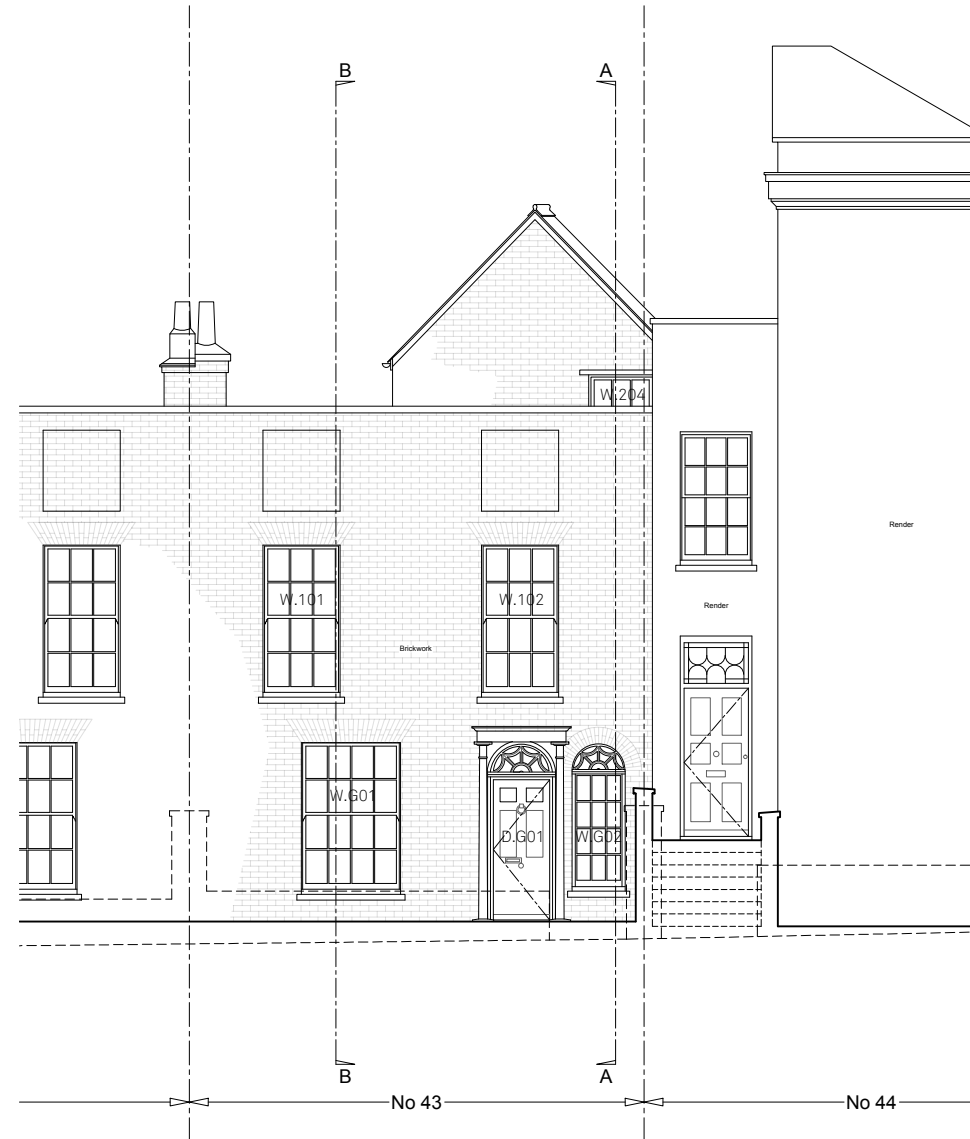
DEMOLITION FRONT ELEVATION 1:100
