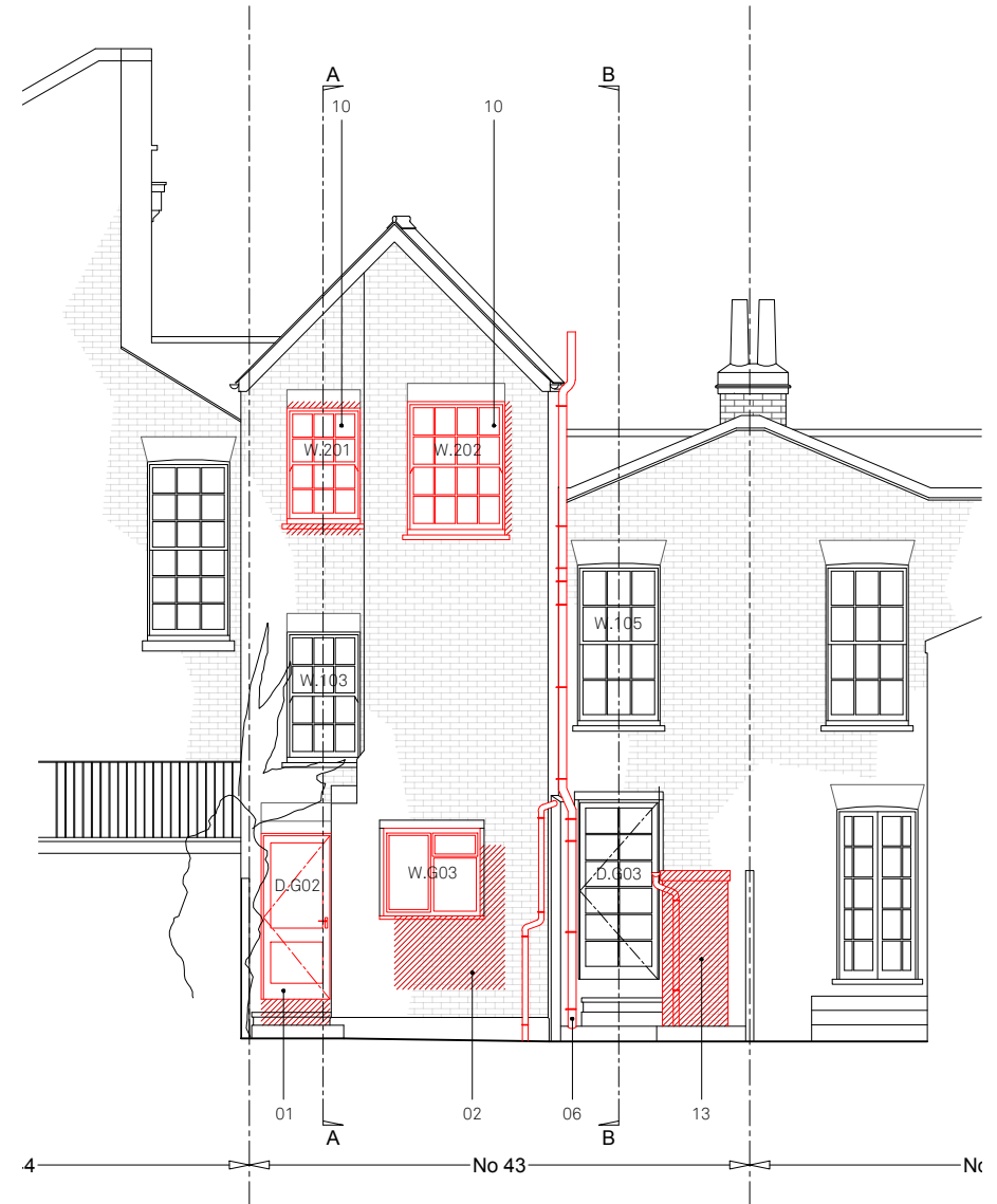
DEMOLITION REAR ELEVATION 1:100
