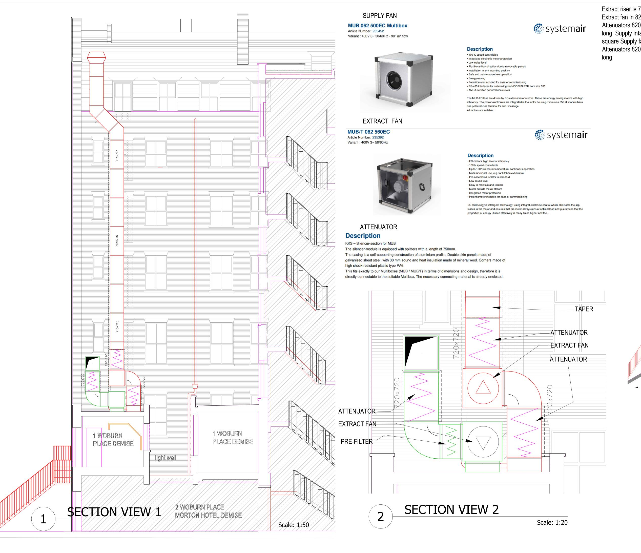
Extract riser is 715mm x 715mm square Extract fan in 820mm square Attenuators 820mm x 820mm x 1020mm long Supply intake is 715mm x 715mm square Supply fan in 820mm square Attenuators 820mm x 820mm x 1020mm MANUFACTURE
