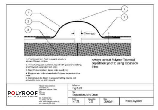
Polyroof pre-formed expansion trims must be fitted strictly in accordance with the Polyroof expansion trim guidance sheet (supplied with trims). A summarised version of the guidance is below for reference.
