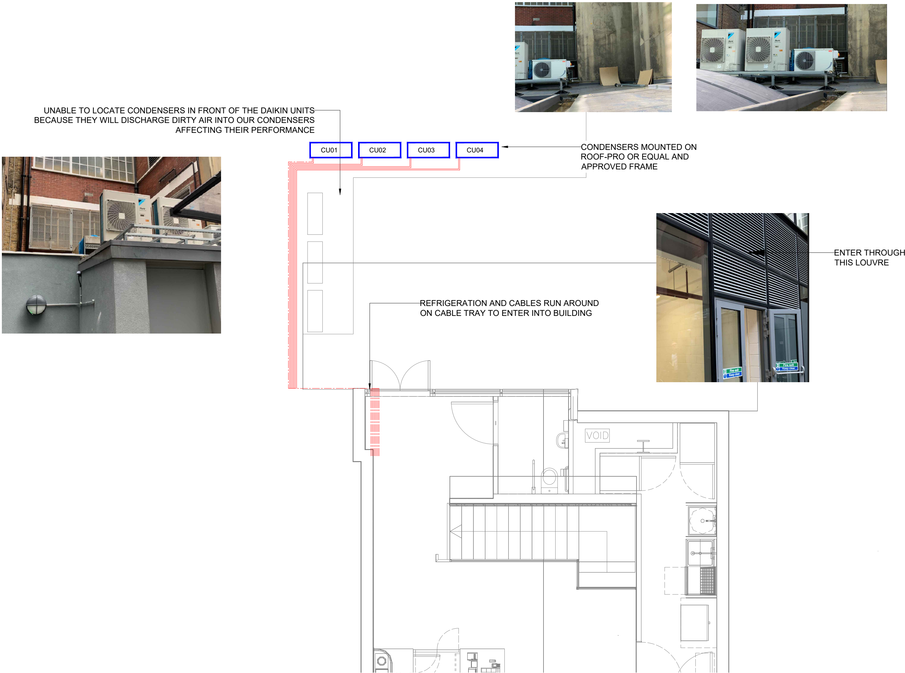
1 GROUND FLOOR - EXTERNAL CONDENSER LOCATION AND REFRIGERATION ROUTE Scale: 1 : 50
