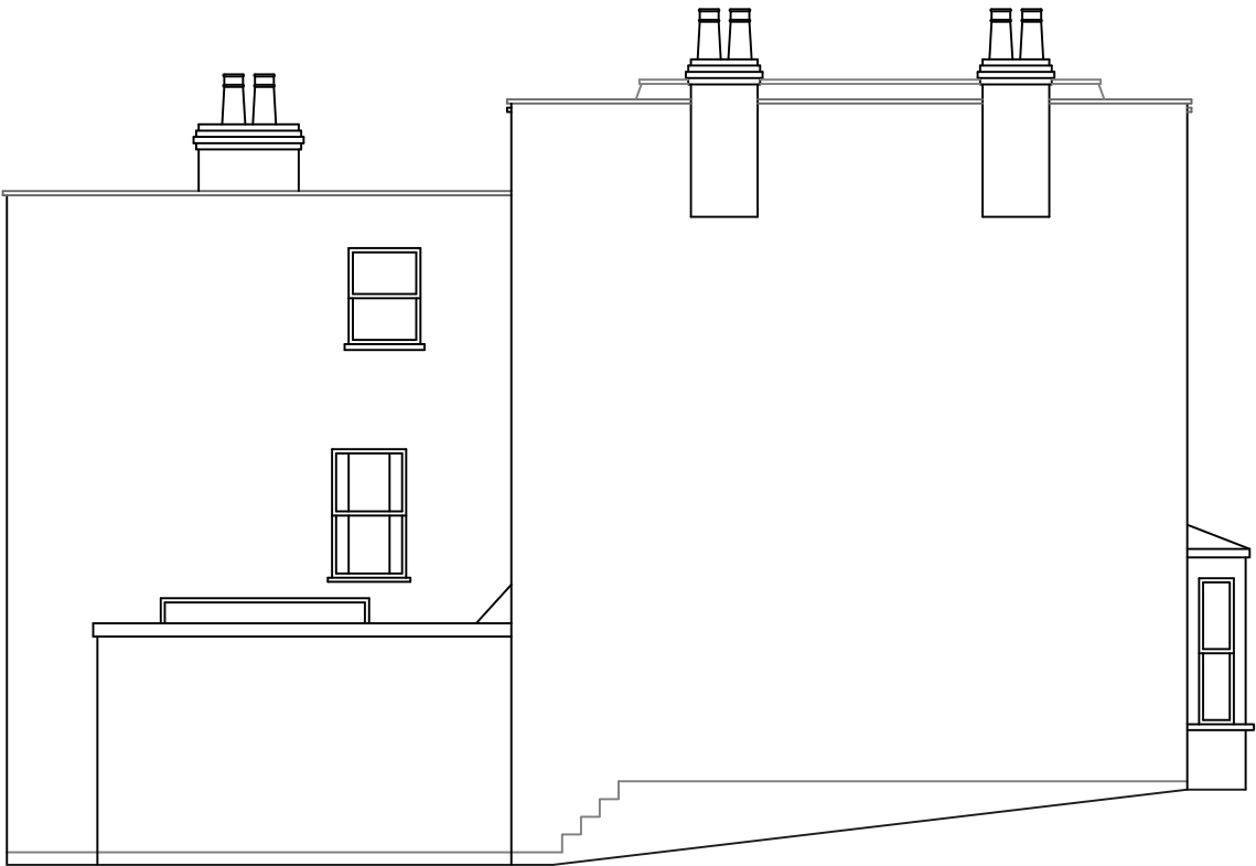
SIDE ELEVATION (EXISTING) SCALE 1:100
