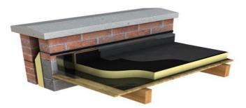
Multilayer Felt System (Bitumem Felt with mineral chippings top layer manufactured by Index
