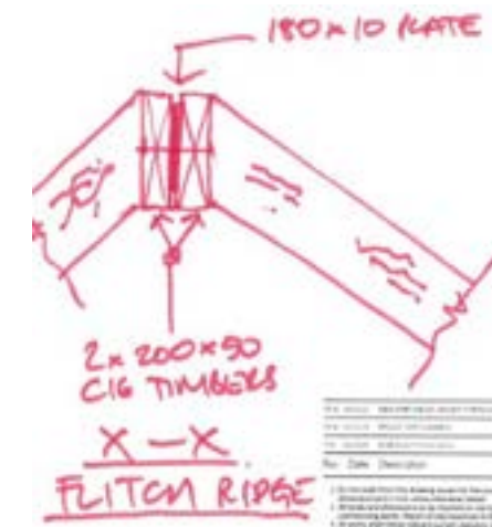
Proposed Recessed Flitch Detail
