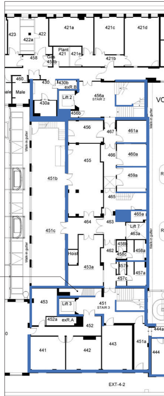
Existing 2018 floor plan of Level 4 with blue overlay indicating original walls remaining
