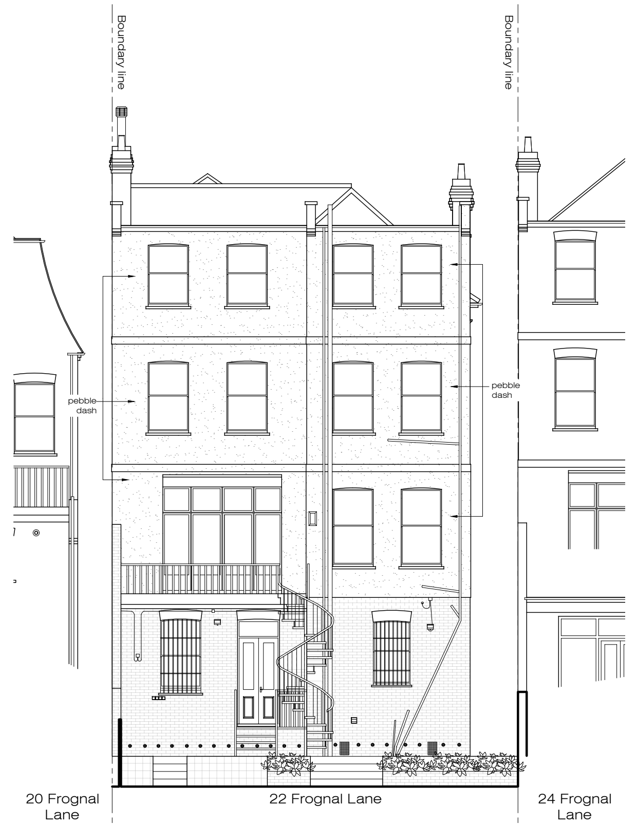
X EXISTING Rear Elevation 1:100@A3
