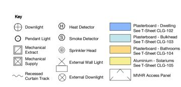
Refer to 35 Series for apartment ceiling details. Service voids and penetrations to be confirmed. Switches to lighting work in progress. Sprinklers required to all units in line with BS standard BS9251:2014. Number and setting out of heads to be reviewed and confirmed by specialist
