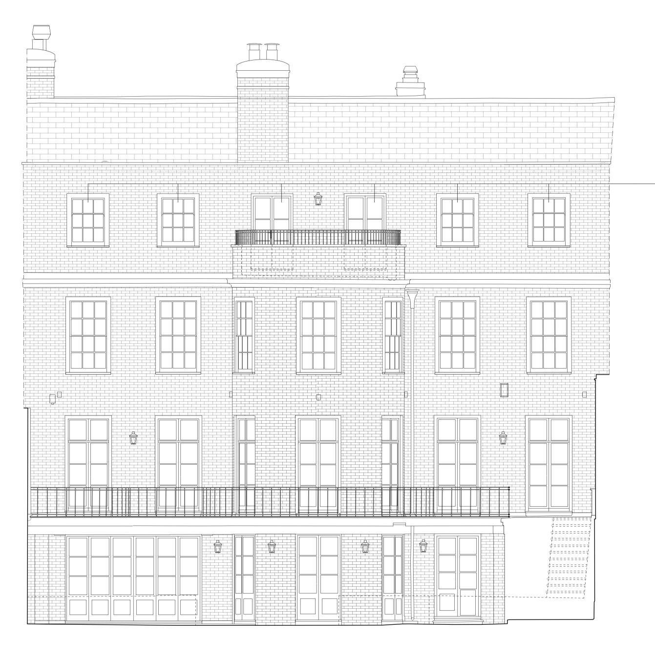
New external doors and windows to match existing on a like-for-like basis, to replace damaged existing set.
