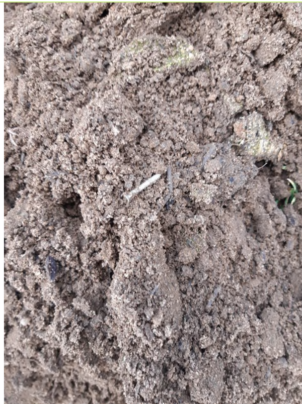
Plate 8: VISIT 27/02/2023 – Remaining soil surrounding remediation zone at TS3 - Orange-brown, silty, fine to coarse SAND with occasional to rare fine to medium gravel of flint and wood fragments and a single metal screw
