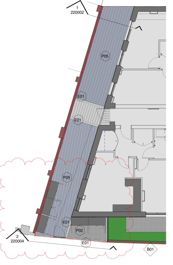
P01(a) - 200x100x80mm Permeable concrete block pavers Bedding layer to Level 0 engineers details 37.500 m -Sub base to engineers details-Membranes to engineers specification
