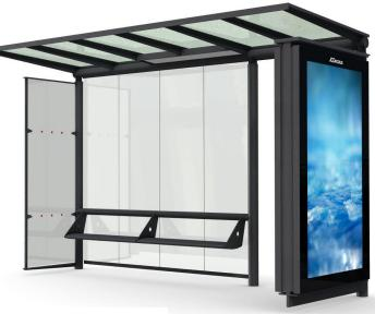
The shelter roof structure is welded steel construction, supporting 5 panels of toughened laminated glass, which cannot fall in the event of breakage The glass is specially treated to reduce the heat of the sun rays by more than 50% and is waterproofed through seals fitted in the glazing bars
