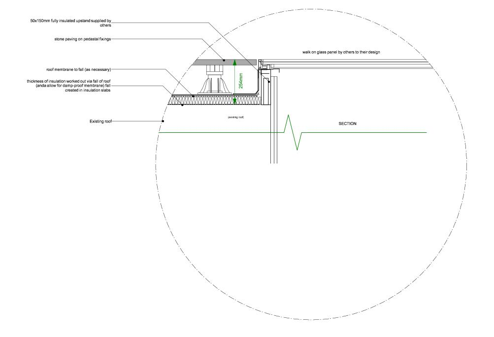
DET 01- Flushed walk on rooflight
