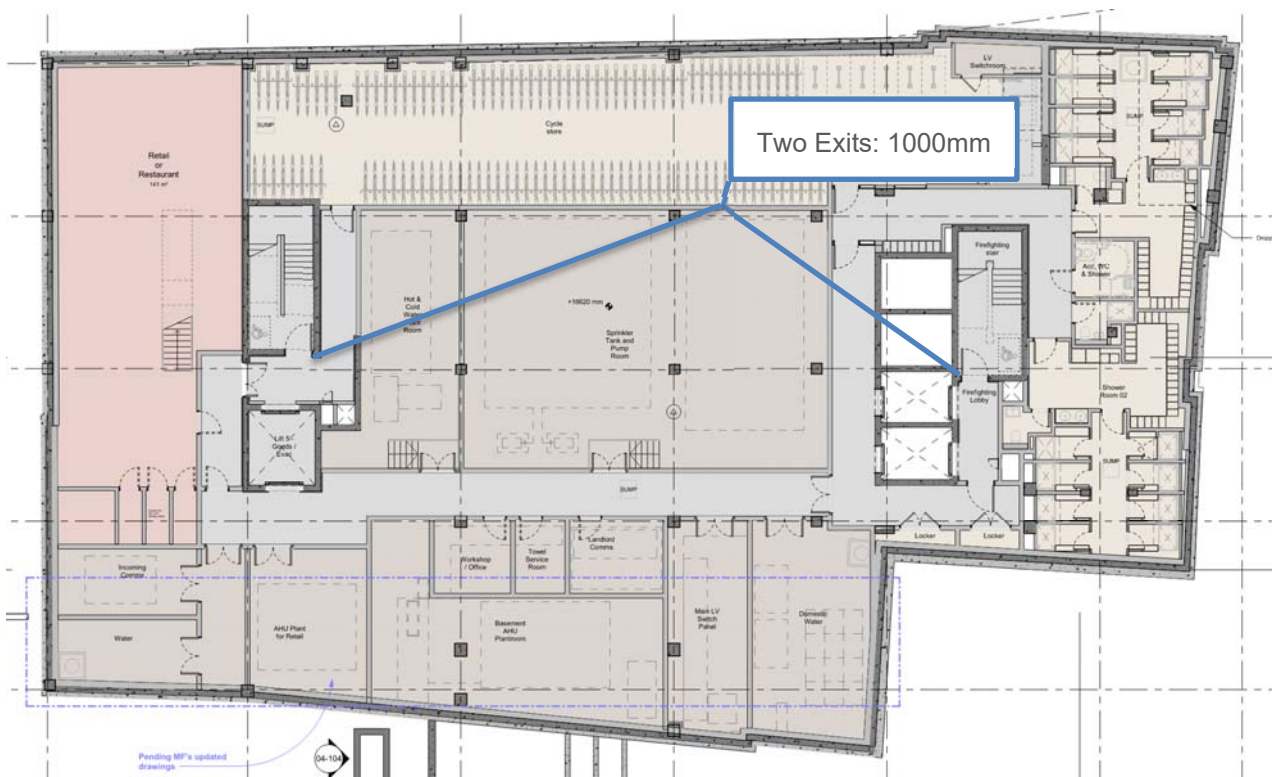
Figure 3: Basement Level B01 horizontal means of escape
