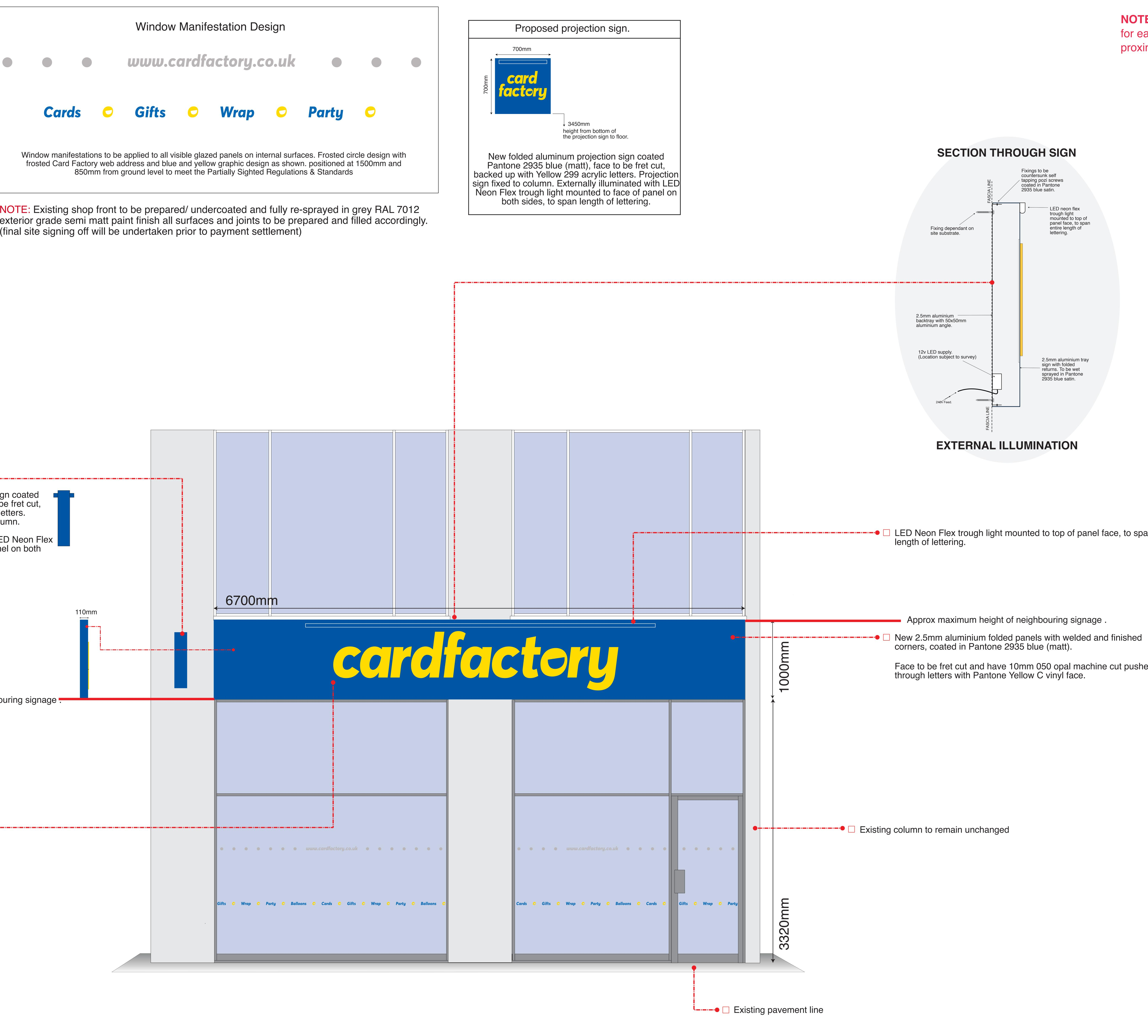
New folded aluminum projection sign coated Pantone 2935 blue (matt), face to be fret cut, backed up with Yellow 299 acrylic letters. Projection sign fixed to existing column.
