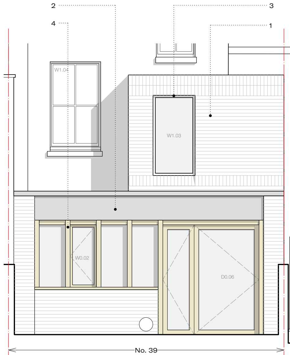
1. New External Brickwork 102.5mm brick with Kalklitr Kalei lime wash paint in 'Cloud'
