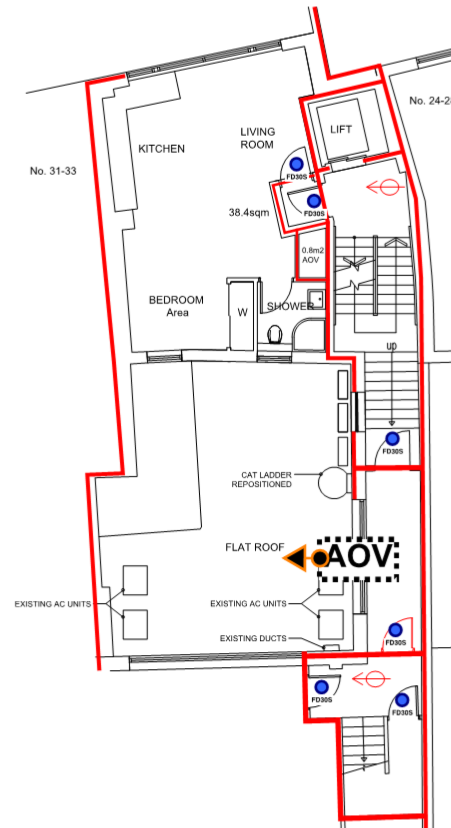
Figure 1: Fire Service Access First Floor
